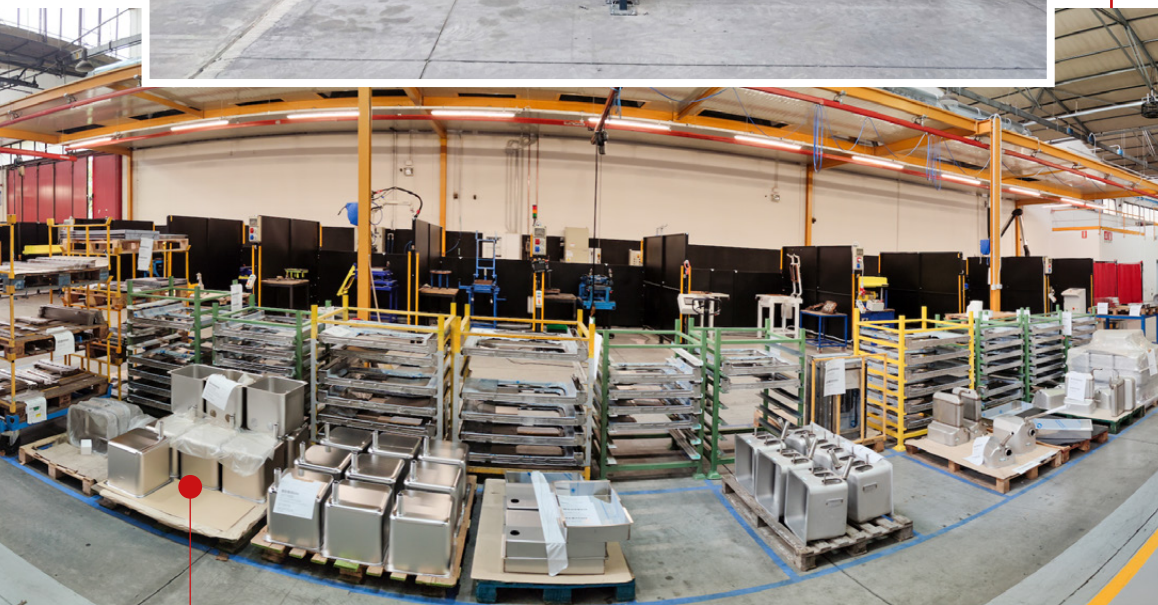
The new Roboteco-Italgargon robotic welding cell installed in Angelo Po moves on a slide of over 20 metres, interfacing itself with 10 workstations
