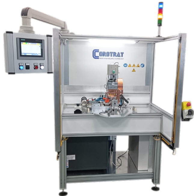
HC 470 G hot-crimping for automated applications for Industry 4.0-5.0
