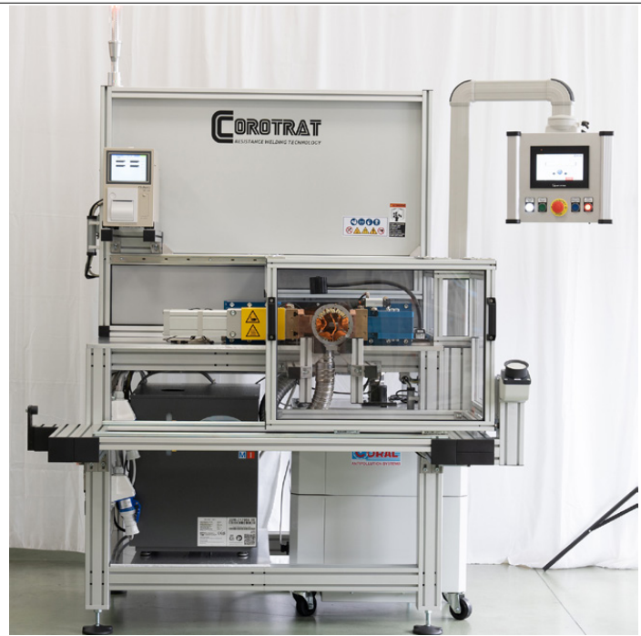
Corotrat's SC35H is a stand alone machine for hot crimping terminals on enameled and insulating wire
