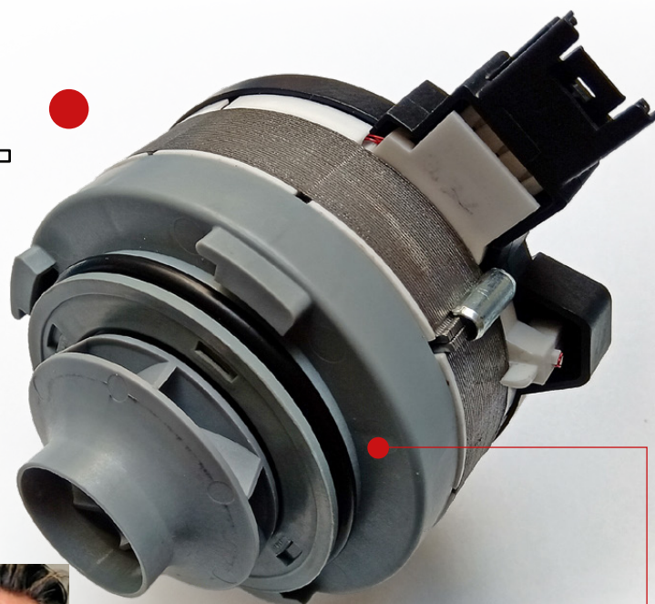
The recirculation pump with three-phase synchronous motor that can be supplied by Askoll according to customers' precise specifications, can be configured with a power that can reach 40 W Hidr and it can be provided with integrated heater, too
