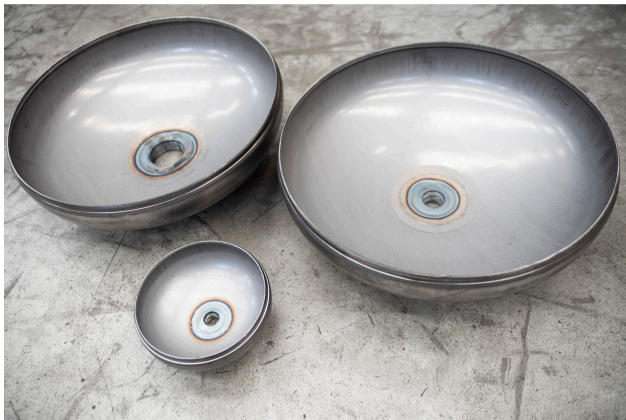
Blanked, drawn, flanged and welded tank bottoms.
