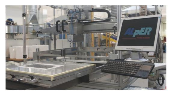
Alper production relies on highprecision printing machines able to assure with accuracy the sizes of the deposited tracks, thickness included
