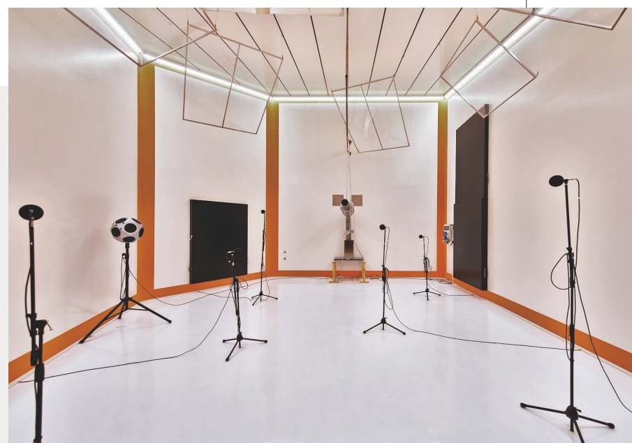
The reverberation chamber of EPL allows carrying out sound power tests in an inner volume of 250 mc and it is characterized by a background noise of just 6 dB.
